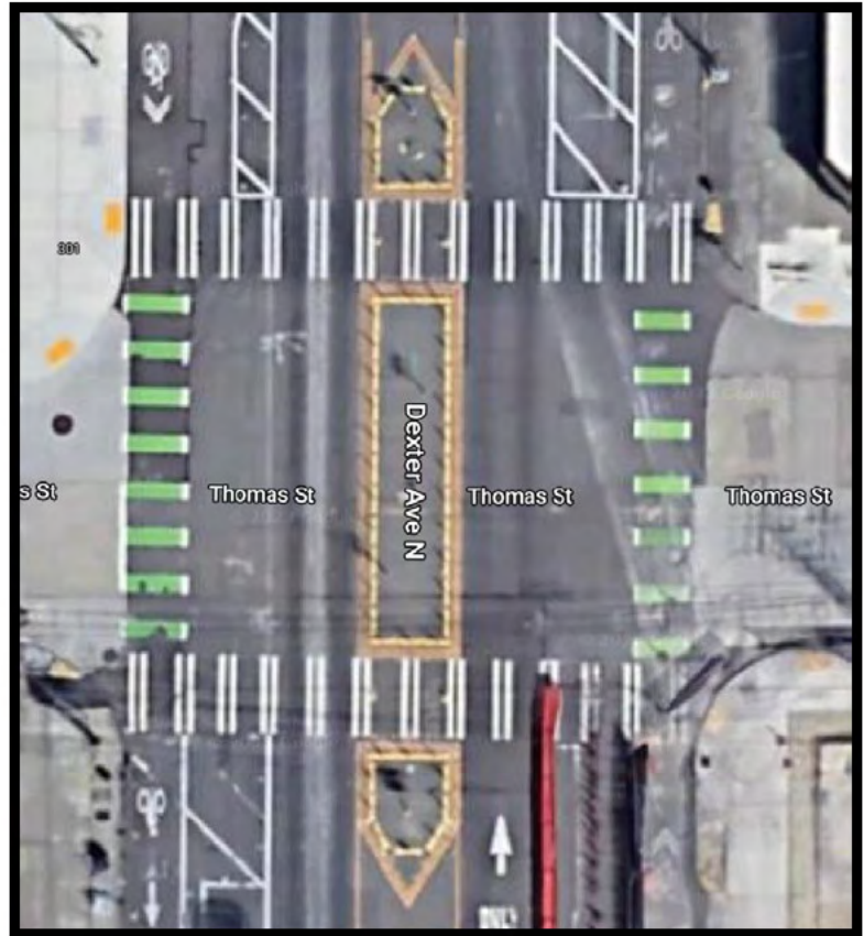
Google Maps overhead view of the intersection. Yellow areas had pylons affixed to roadway.
